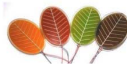
Leaf-shaped transparent DSC with four colors courtesy AISIN SEIKI CO.,LTD.
